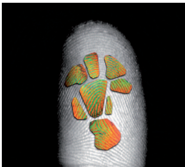
Figure 20. A full-color fingerprint visualized using an elastic photonic crystal, overlaid onto a grayscale image of an index finger. From Ref. [213].
